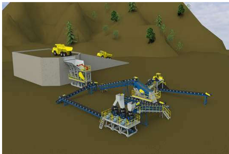
Sepro System: 75t 3 Stage Crushing Circuit
