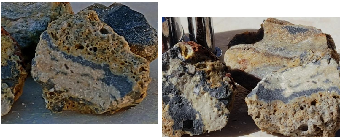
Figure 6 AC hole 5100-1 showing chalcedony with sulphides at 92m down hole
