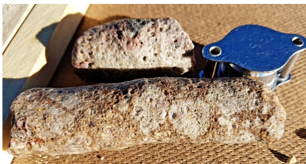
Figure 5 AC hole 5100-1 showing silica alteration at 30m down hole (top left), silica-alunite at 36-37m (top right), and brecciated silicified rock with alunite matrix-mosaic-jigsaw breccia at 39m (bottom).
