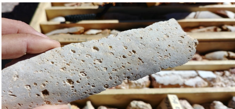
Figure 4 Core sample from diamond drill hole 5300-2. Alunite-rich vuggy silica intercept from 46 to 50 metres down hole.
