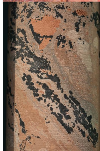
Cobalt oxide mineralisation (black) in diamond drill core
