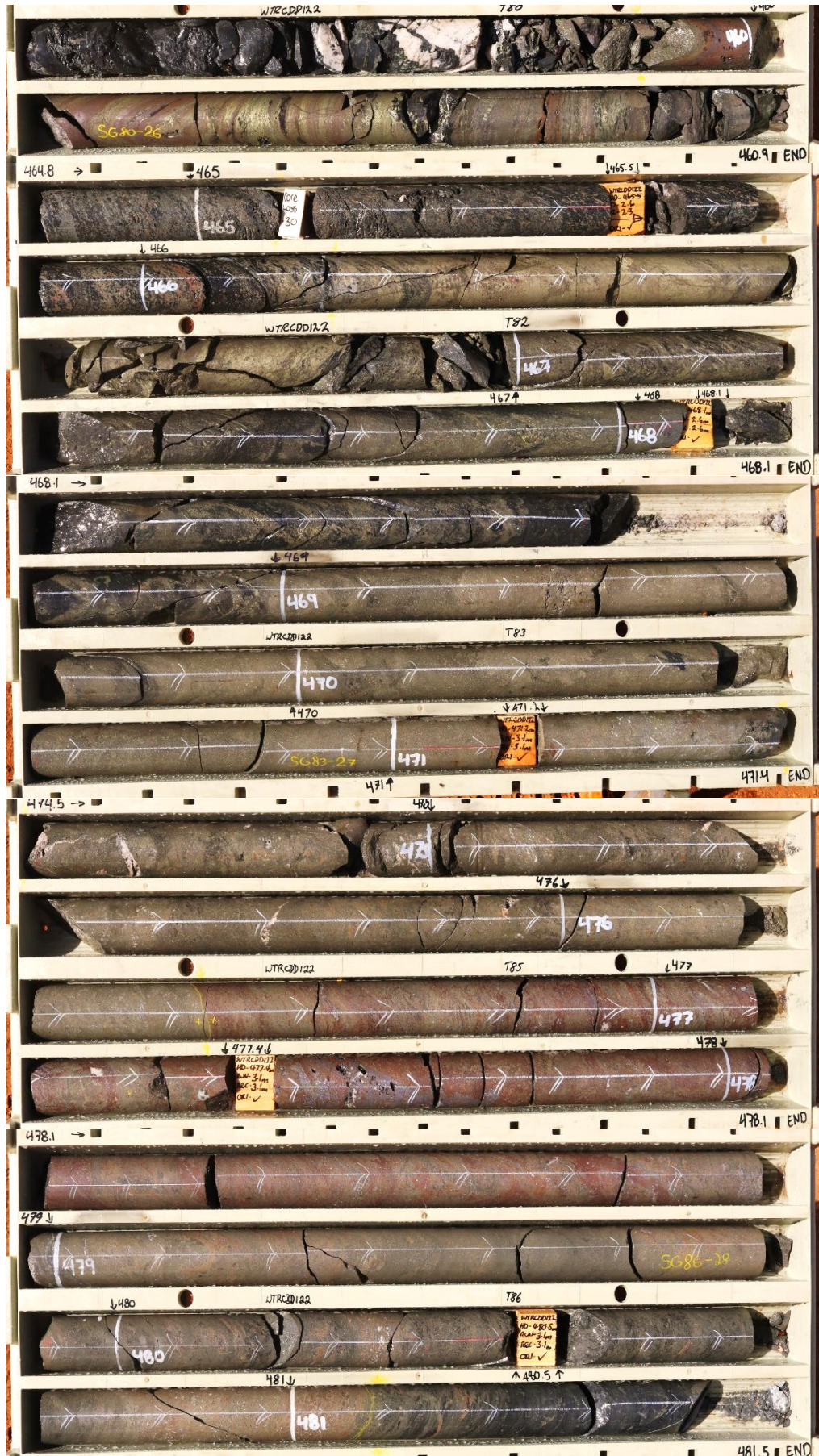
Figure 1 - WTRCDD122 Highlights: Massive/Semi-massive pyrite-sphalerite-galena-chalcopyrite
