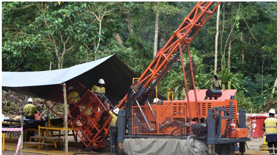
Photo: Diamond drill rig set up underway at Misima Gold Project
