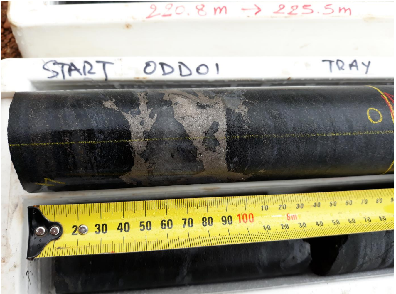
Image One | Sulfides containing Nickel & Copper in the first drill hole at the Odin Prospect.
