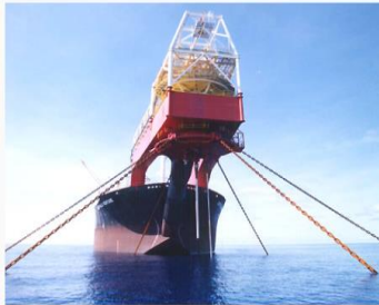
The FPSO, showing the single-point mooring.
