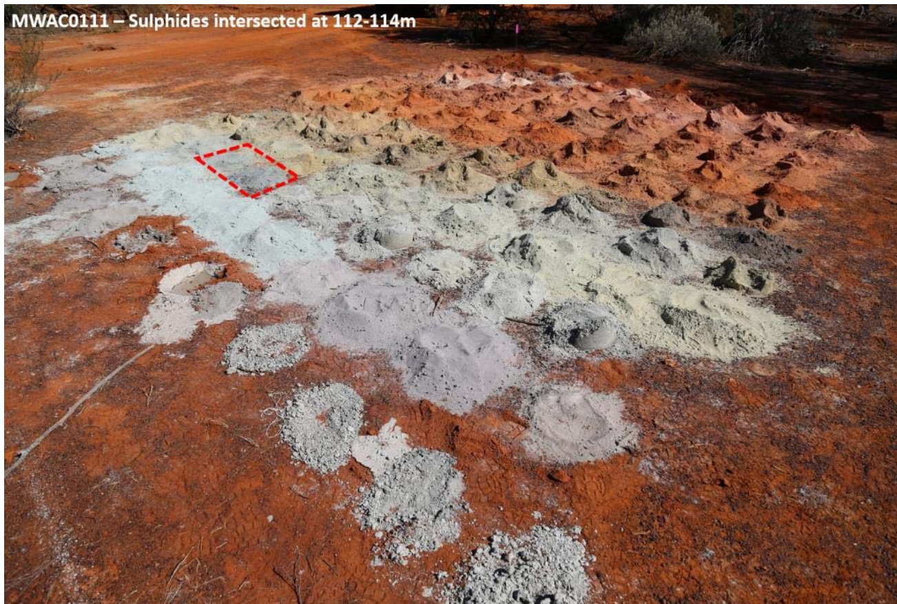
Figure 7: Aircore drill spoils from MWAC0111 showing sulphides intersected at 112-114m.
