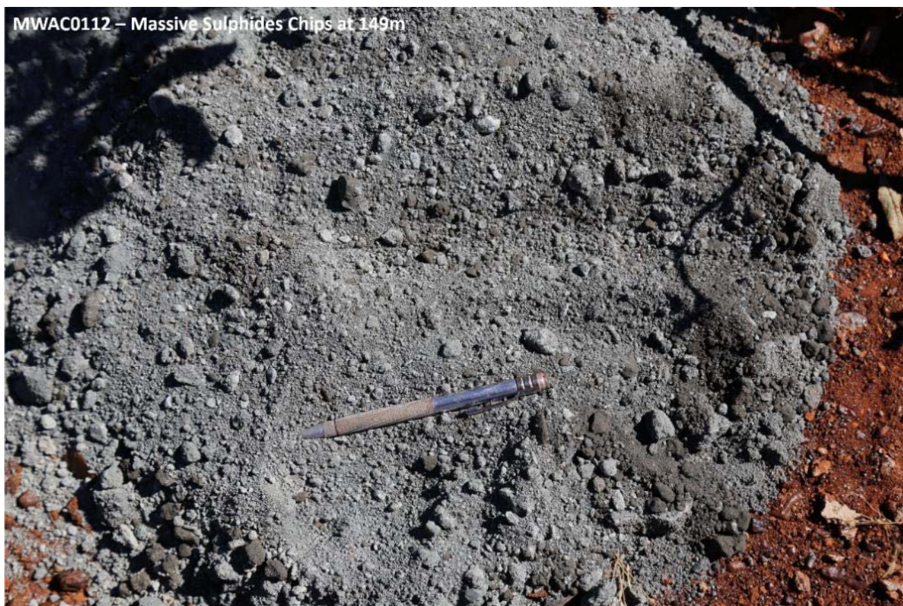
Figure 10: Aircore drill spoils from MWAC0112 showing massive sulphides chips, pyrite and minor chalcopyrite at 149m.
