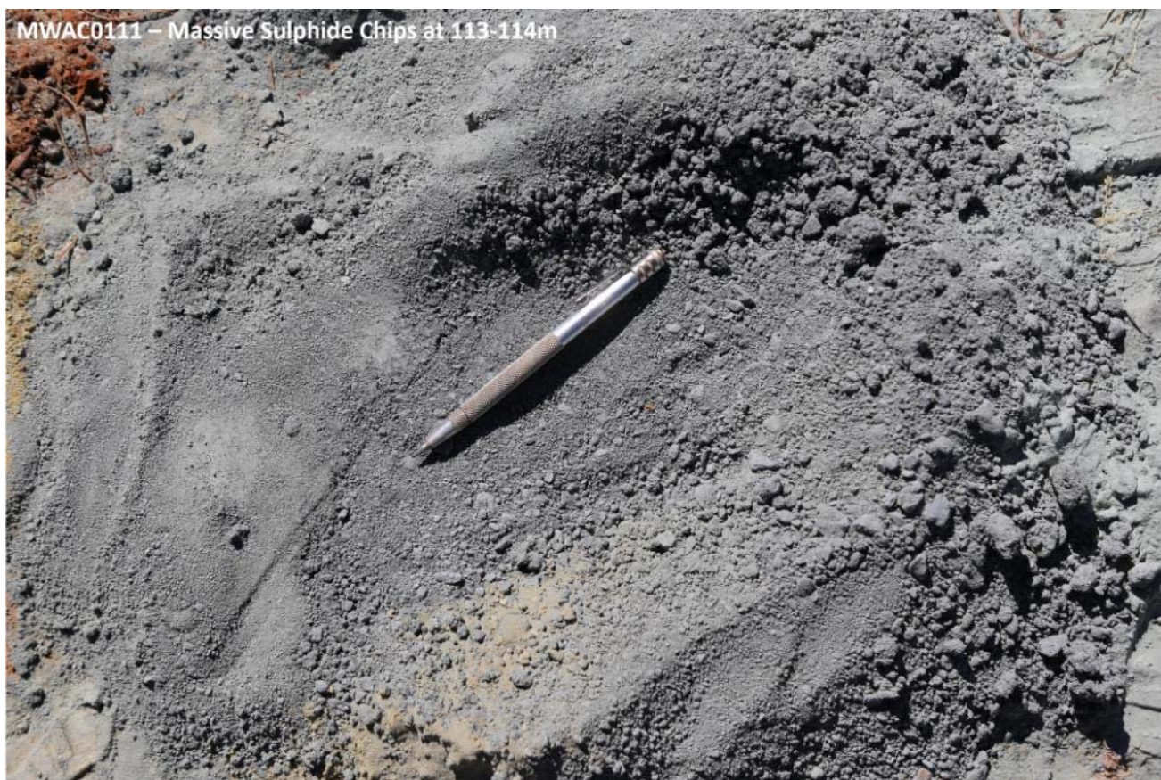
Figure 8: Aircore drill spoils from MWAC0111 showing massive sulphide chips, pyrite with minor chalcopyrite at 113-114m.
