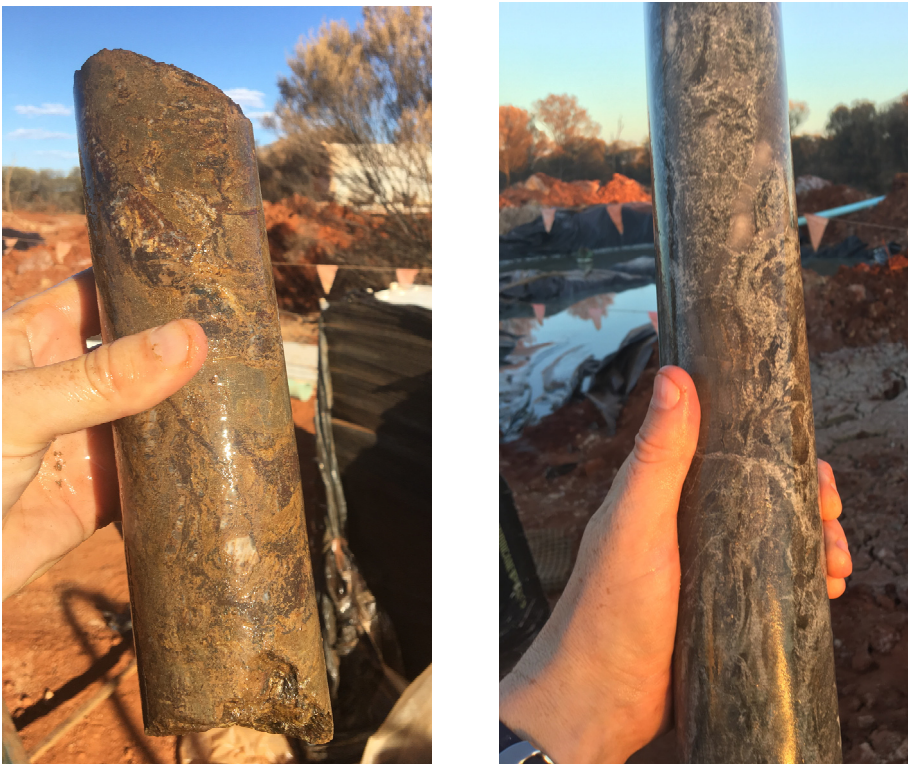
Figure 5: 18CWDD0037 drill core photos showing strong biotite alteration with quartz-carbonate veins and pyrite-chlorite-silica alteration in the steep-dipping, north-west oriented structure. The photo on the left is of variably oxidised altered/veined rock and taken from 80m down hole, while the photo on the right is of fresh altered/veined rock and taken from 134m down hole. Note visible gold was seen in quartz veins at 59m and at 126m down hole. Assays are pending.
