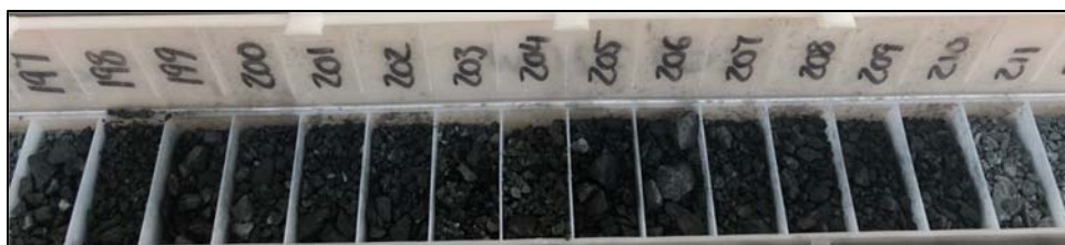
Figure 1: Zone of massive and semi-massive sulphide in a silica-rich unit (probable exhalite) in MURC002; zone correlates well with the DHEM modelled plate position.
