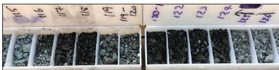
Figure 2: Pulses of massive and semi-massive sulphide in silica-rich units in MURC001 surrounded by highly altered volcanics; also correlated well with the DHEM plate position.
