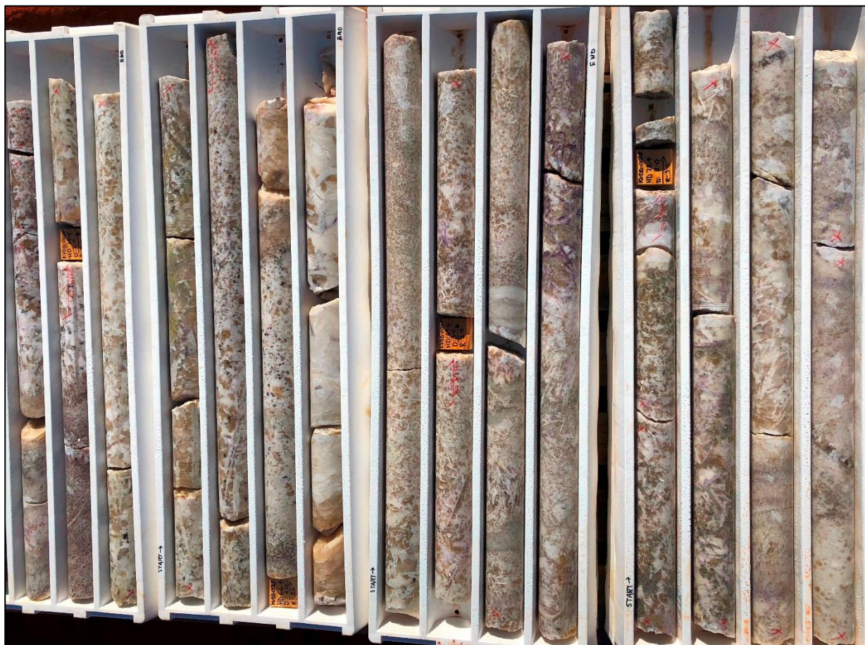
Figure 5: Kathleen's Corner– Diamond core hole KVDD0002 showing wide pegmatite zone (Trays ~ 1m long)
