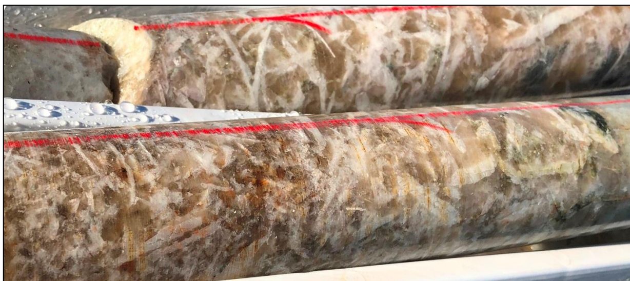
Figure 6: Kathleen Valley– HQ drill core (64mm diameter) showing coarse white spodumene crystals
