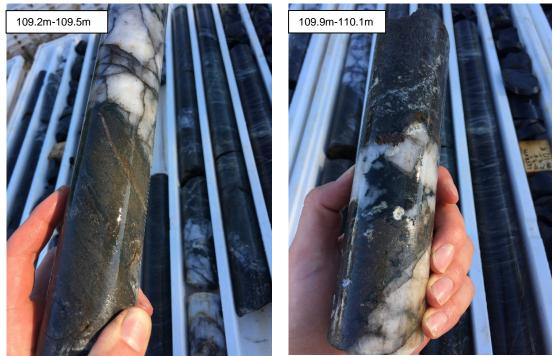
Figure 2 Examples of quartz veined sulphide altered BIF from diamond hole LEFR074
