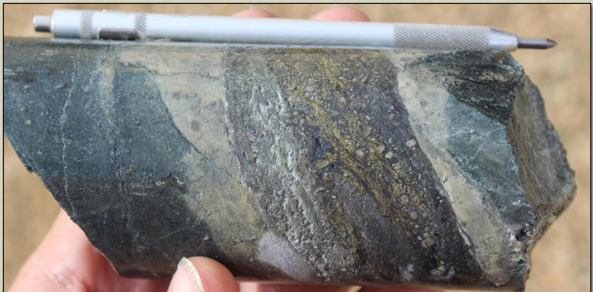
Photo 4. Pyrite-chalcopyrite-chalcocite D vein at 151.9 metres in SMD025.
