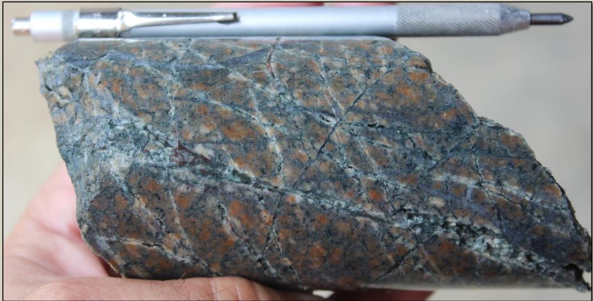
Photo 5. Quartz-magnetite ± hematite 'M' veins in a hematite altered quartz-diorite porphyry at 272 metres depth in SMD025.
