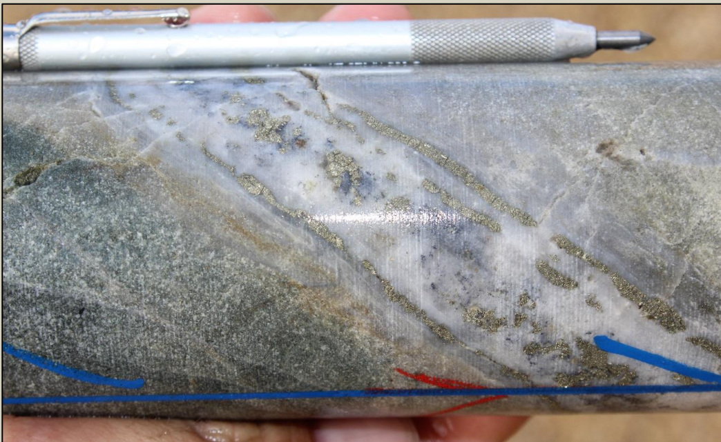
Photo 1. Quartz-pyrite-molybdenite porphyry 'D' vein at 332 metres depth in SMD024.
