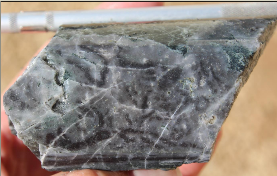
Photo 3. Quartz-magnetite-pyrite-chalcopyrite M veining at 441m in SMD024. Note the 'wormy' nature of the M veins having similar character to porphyry A veins which are likewise part of the earliest vein phases in a porphyry.
