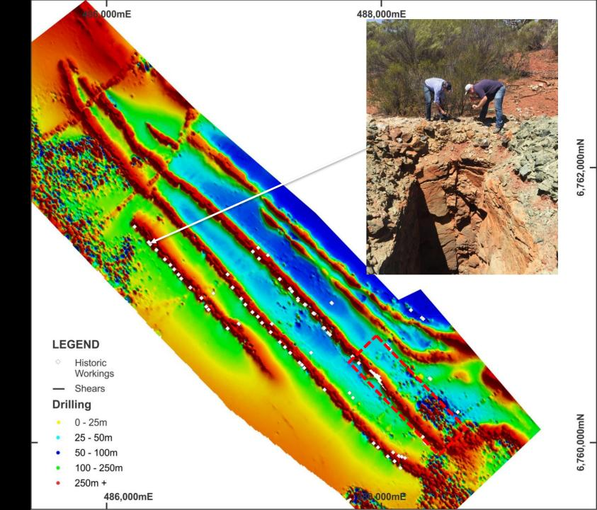
A detailed ground magnetic survey was undertaken in 2017, the results demonstrated that the historic workings were positioned on the footwall and hanging-wall contacts of the 3 parallel ultramafic units (depicted by the dark red contrast). The survey also revealed for the first time that the potential strike as indicated by; previous historic workings, the current Mineral Resource Estimate and the interpretation of the ground magnetic survey - demonstrate a potential strike length of 14km.
