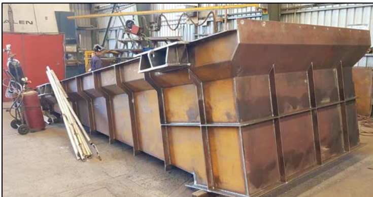
Figures 19 & 20: Offsite pipework and equipment fabrication for Century Processing Plant refurbishment
