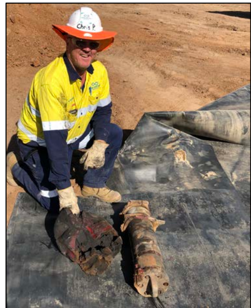
Figures 21 & 22: Initial pipeline 'hot tapping' for localised draining, controlled removal and capture of water (left) and Process Plant & Pipeline Superintendent Chris Portelli with the extracted cleaning pig (right), allowing for water commissioning activities to begin in June
