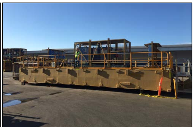
Figures 9 & 10: Design of the Water Winning Pontoon for extraction of feed water from the Evaporation dam (left) and fabrication of the pontoon in Perth nearing completion for June delivery (right)
