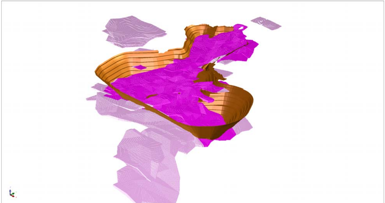
Figure 2: Oblique View of New Pit Design (dark magenta = Indicated, light magenta = Inferred, mineral resources)
