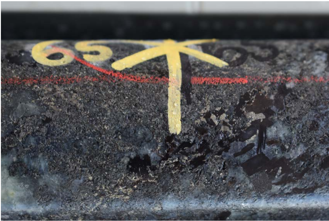
Figure 6. Gold bearing sulphide mineralisation intersected in A8RC005 near gravity Anomaly 9.
