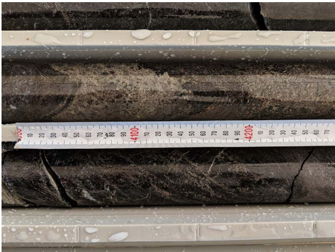
Figure 7. Massive sulphide mineralisation associated with nickel and cobalt in ultramafic gneiss in A8RC011.
