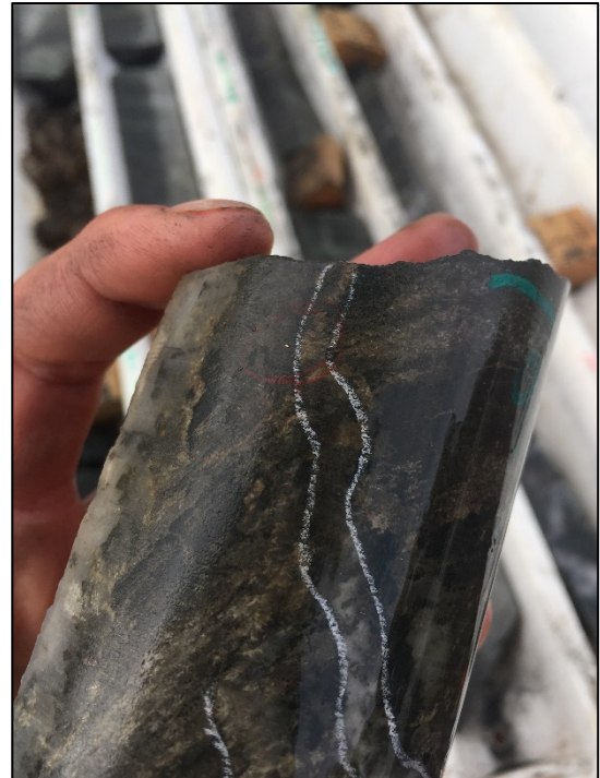
Figure 2. Visible gold on margins of quartz vein within strongly sulphide replaced BIF in hole LSRD009 – 89.7m
