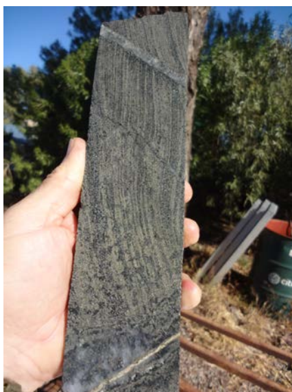
Figure 7. Sulphide replaced BIF from core hole LSRD009-64.6m-64.8m
