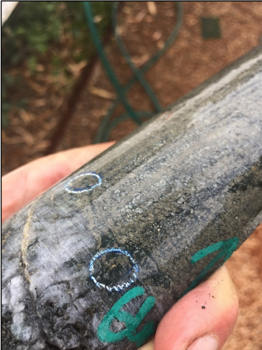
Figure 1. 2x specks of visible gold on margins of quartz vein within strongly sulphide replaced BIF in hole LSRD009 – 64.4m
