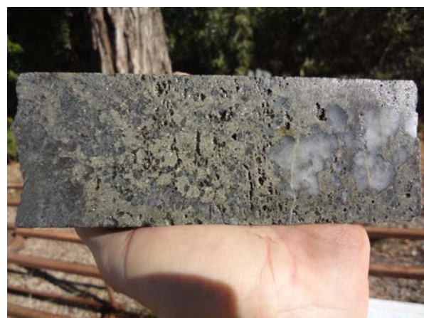
Figure 8. Strongly sulphide replaced BIF from core hole LSRD009-83.8m-83.98m
