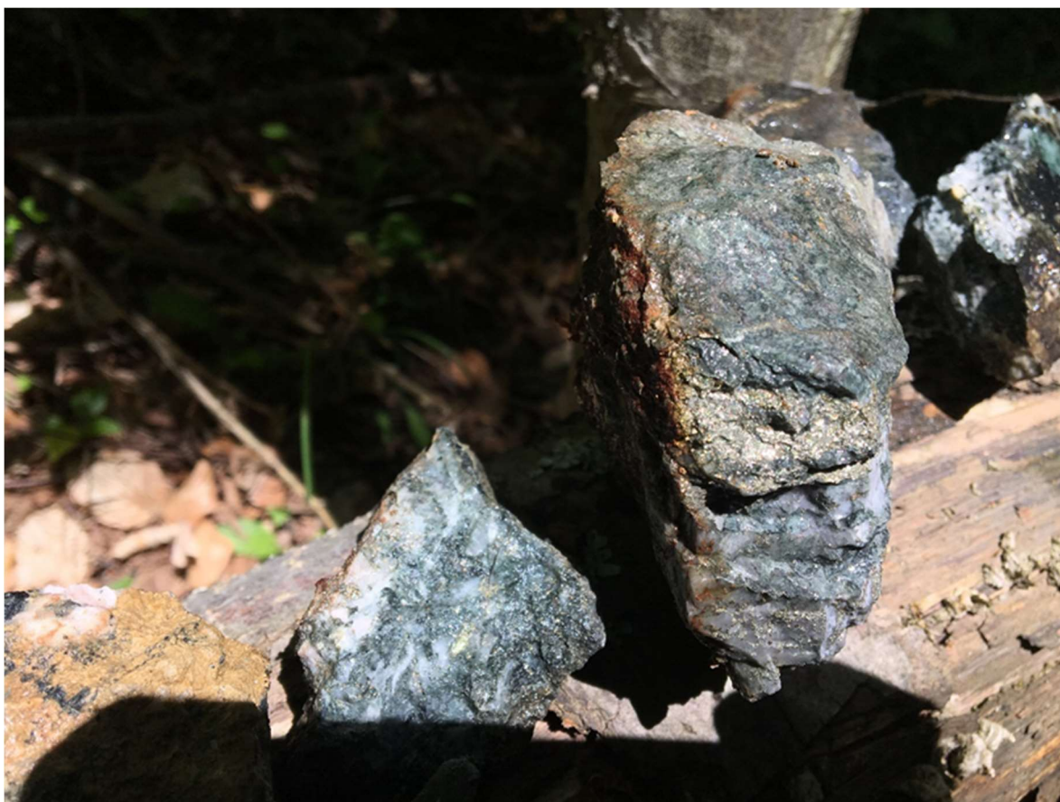
Figure 7 – Sample Sp10021, was collected from stockwork zone, which is located over the interpreted IP anomaly between IP lines AA and B. The sample is highly silicified and contains pyrite and chalcopyrite mineralisation.
