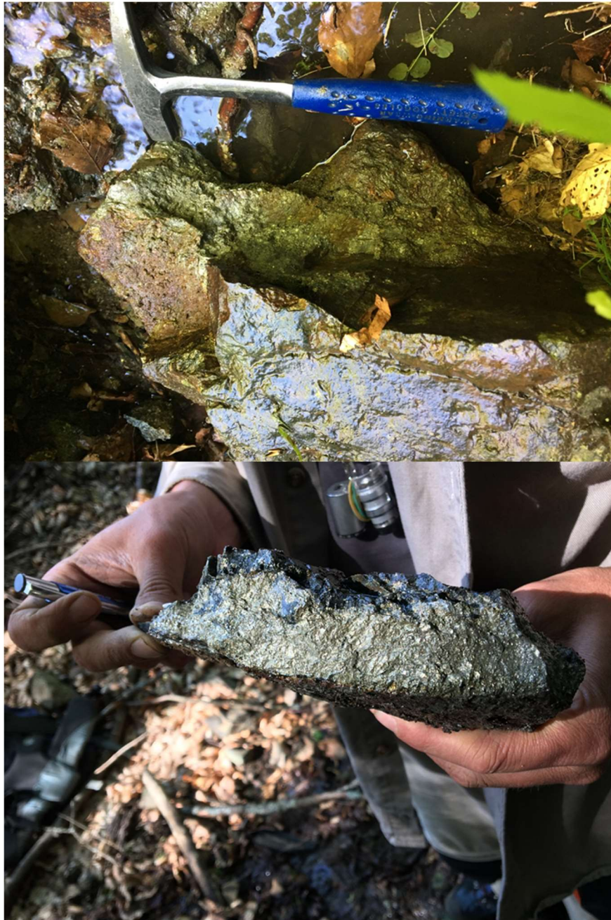
Figure 6 – Sample SP10019 was collected from a quartz vein and is located over the interpreted chargeability anomaly on line C. The sample is comprised of massive sulphide mineralisation (Pyrite and traces of Chalcopyrite), and silicification
