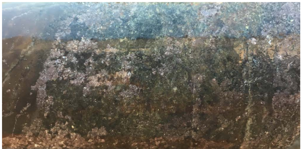
MIDD010 at 40.2m, within a 1m interval of 1.85% Co and 0.42g/t Au
