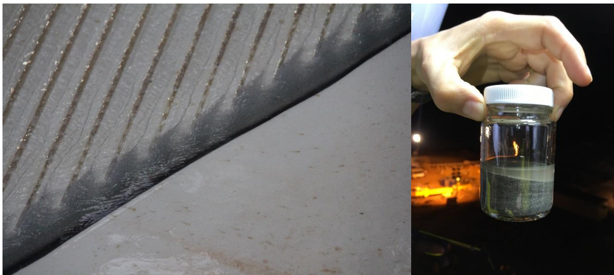
Tantalite Concentrate on the Wet Table (Photo 2) and Final Primary Tantalite Concentrate (Photo 3)
