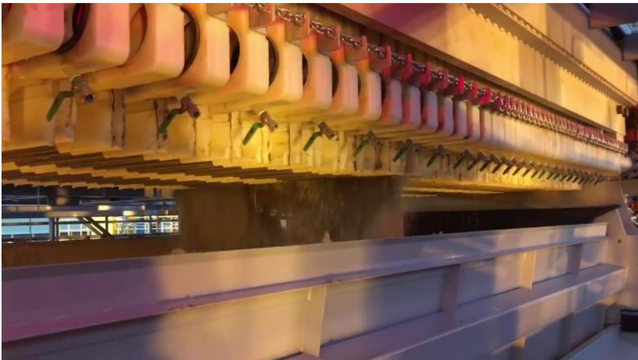
Fines Spodumene Concentrate Discharged from the Filter Press at the Pilgangoora Project (Photo 1)
