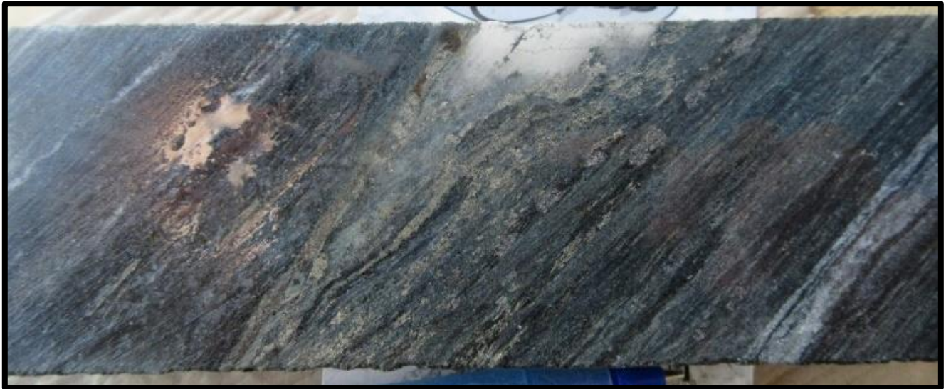
Figure 1. Image of drill core showing an example of the Iron Formation with sulphides from drill hole KAS-18-03.
