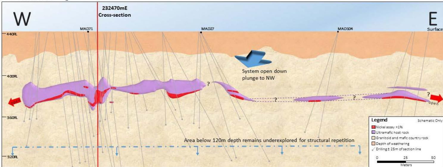
*Above: Schematic cross section of the MAD71/MAD85 line (facing west) at Stricklands based on drill hole data. The mineralised ultramafic dips to the north-west with potential for a down plunge extension. Left: long section of Stricklands highlights the multiple intersections of +1% Ni mineralisation over a 400m strike.*
