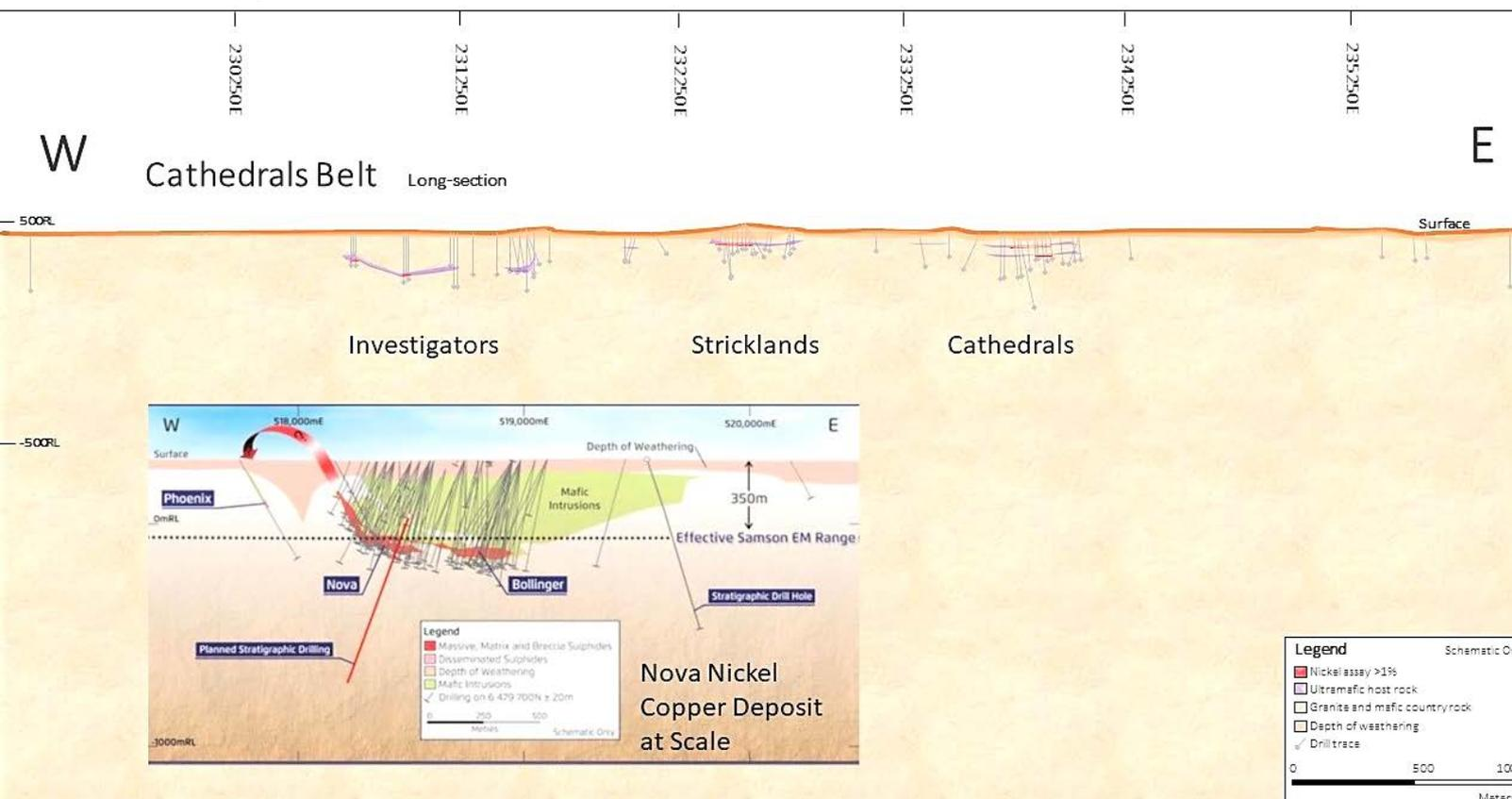
*Left: Schematic diagram of the Cathedrals Belt (based on drill hole data to date) shown at the same scale as the Nova deposit in the inset diagram (Nova Ni resource of approx. 270,000t contained Ni). The comparison shows the longer strike of mineralisation at Cathedrals with large areas untested along strike and at depth. Nova shown as scale and an exploration stage comparative, not as a direct analogue.*
