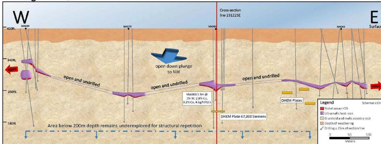
*Above: Schematic cross section of the MAD60 line (facing west). The mineralised ultramafic dips to the north-west with potential for a down plunge extension, where the new 67,000S EM conductor is located. Left: long section of a 1,000m portion of Investigators highlighting the multiple intersections of +1% Ni mineralisation and the new EM conductors to be drilled.*
