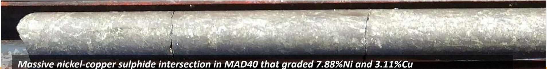
*Massive nickel-copper sulphide intersection in MAD40 that graded 7.88%Ni and 3.11%Cu*
