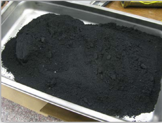
Figure: Graphite product unloaded from the reactor (left) and XRD analyses confirming the graphitic nature of the product (right).
