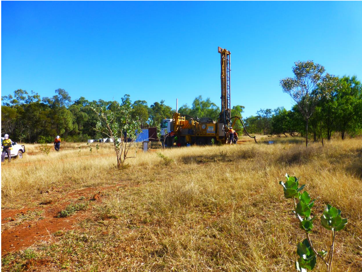
Figure 1: Australian Mines' Mineral Resource expansion drilling has now commenced at its 100%-owned Sconi Project in northern Queensland. This reverse circulation (RC) drill program comprises approximately 50,000 metres of drilling and is designed to extend the mineralisation of the three deposits that form the Company's Sconi Project.
