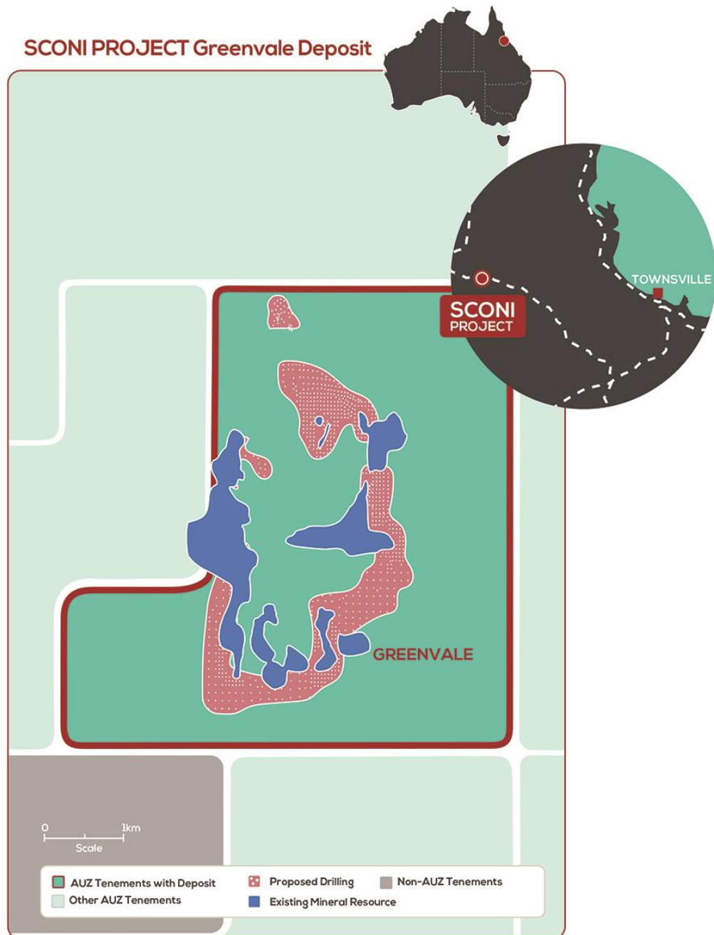
Figure 2: The Greenvale deposit - one of three deposit that comprise Australian Mines' Sconi Project. Areas of the proposed Mineral Resource expansion drilling are shaded in red. Outline of the current Mineral Resource is shaded in blue. The Greenvale mine complex contains multiple zones of cobalt and nickel mineralisation within Australian Mines' 100%-owned granted Mining Lease. The majority of these cobalt and nickel zones have only been sparsely drill tested and mineralisation remains open to extensional drilling. Australian Mines believes higher grade ore may still be available to add to the existing Mineral Resource, with the zones being targeted with this program showing strong potential.
