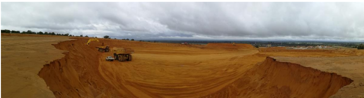
Photo 2: Overburden Removal at Boonanarring (27 June 2018)
