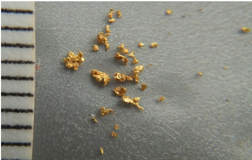
Figure 1. Gold panned from ~3kg air core sample from 16-17m in TGGAC181: scale at left in mms.
