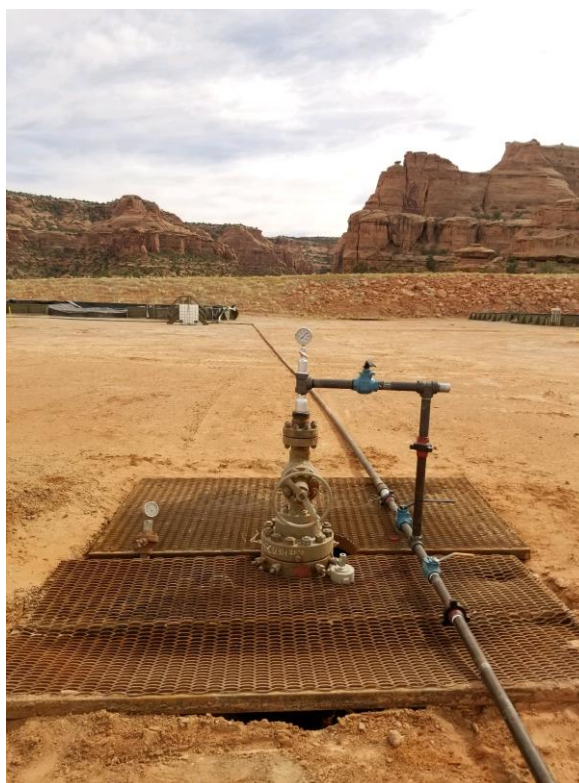
Figure 2: Well head setup so both bulk samples and small samples can be collected.
