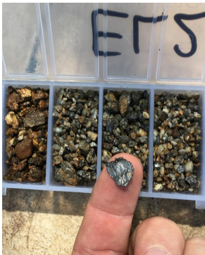
Figure 4: Example of the graphite mineralization observed in follow up drilling around significant intercept from EL258A. Approximate width of flake is 10mm.
