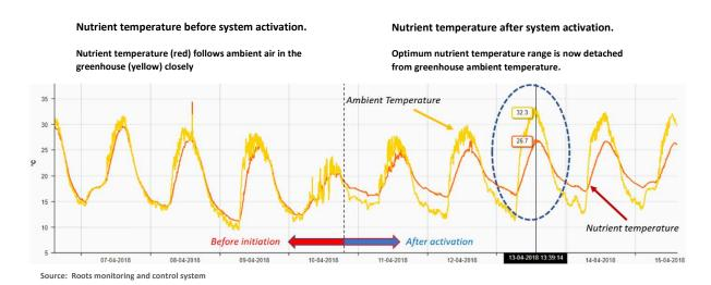
However, using the RZTO and NFT system, the farmer was able to stabilise and monitor the plant roots to ensure they remained at an optimum temperature, irrespective of the greenhouse's ambient air temperature."
