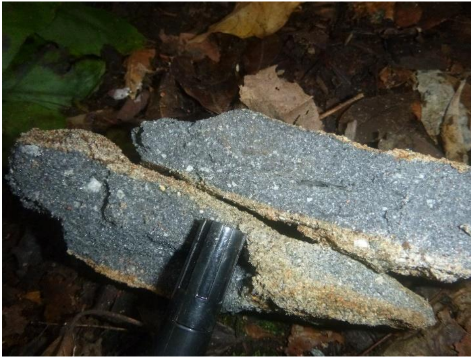
Sample MKR160B from Dikaki – Sphalerite and galena bearing sandstone – returned an assay of 29.8% Zn+Pb
