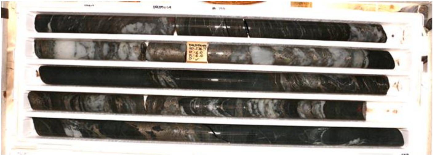
Figure 4a: Photo of drill core hole DRDD059 4.3 m @ 8.8 g/t gold from 575.3 m including 3.4 m @ 10.4 g/t gold from 576.2m and 0.3m @ 44.4 g/t gold from 584.3 m
