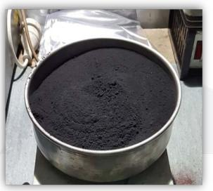
Photo 1 : Single run graphite produced from the Hazer Process
