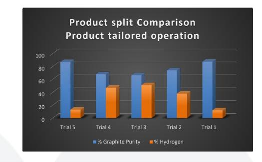
*Graph 2 : Comparison of hydrogen/graphite purity achieved per test run.*
