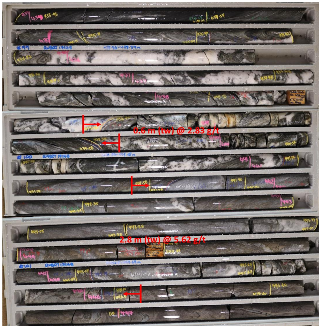
Figure 7 Core photos of significant results in hole RUBRT17148.
