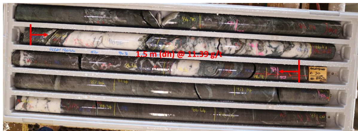
Figure 11. Core section of PEGRT18044 showing new Pode like structure found in drilling for Pegasus K2. Visible gold present in this intersection
