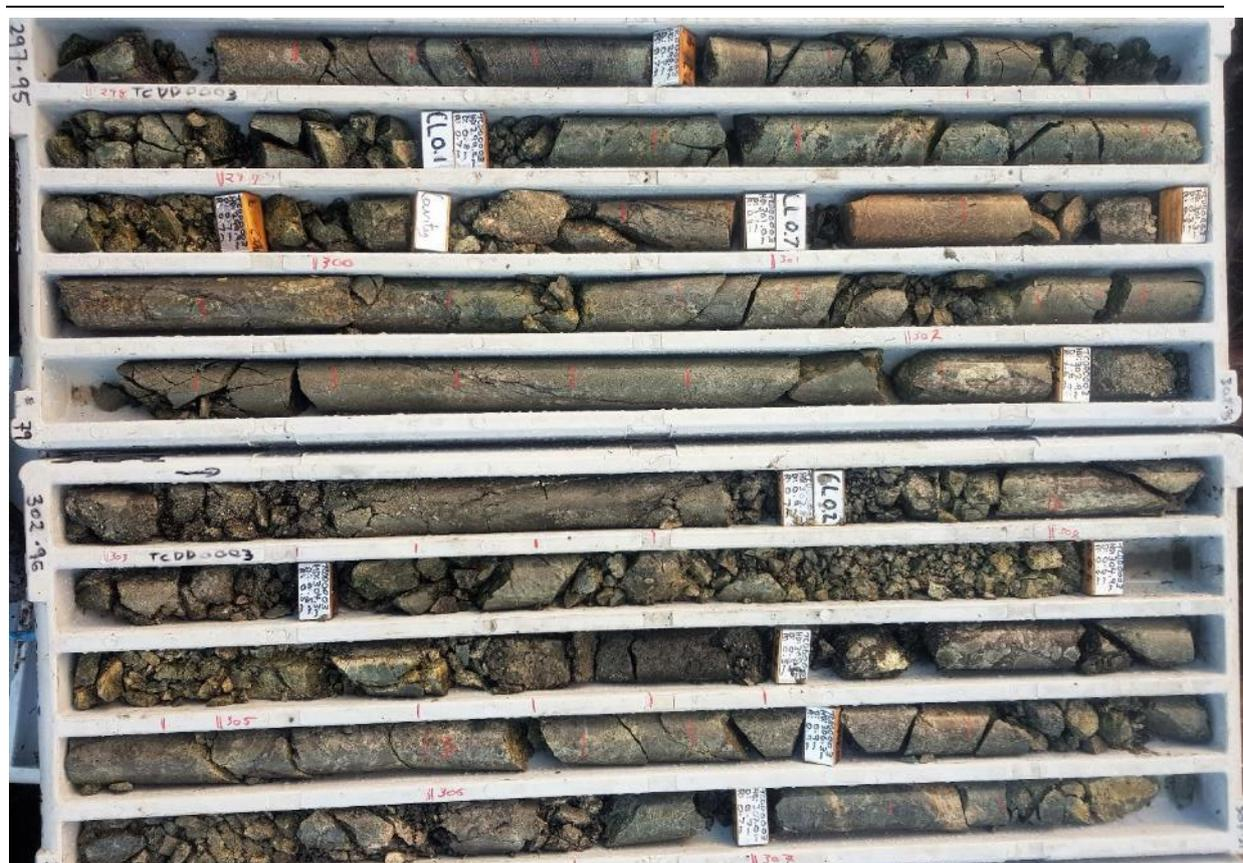
Photo 1: Drill Core TCDD003 297.95m to 307.31m
