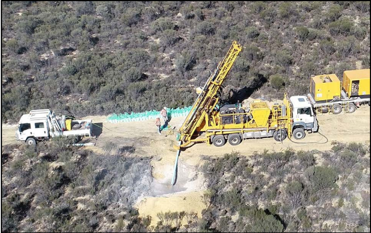
Figure 3: RC drilling earlier this month at Mt Holland West .
