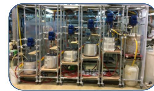
Neutralisation & Precipitation Circuit – Hydromet - ANSTO
