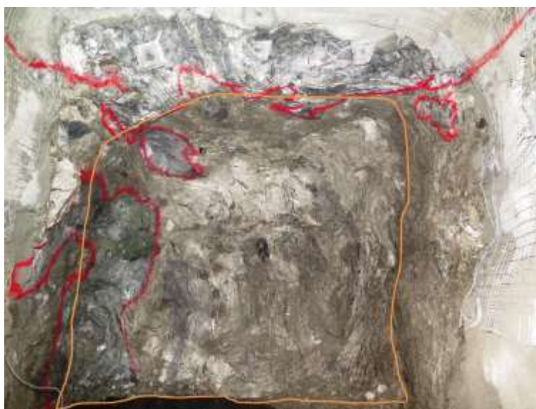
370 S1 ore drive with an average face grade of 7.6% nickel
