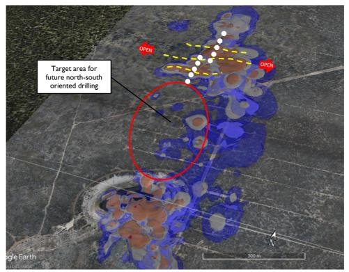
Figure 5: Lady Magdalene (Leapfrog Resource Model) – Showing drill holes (white) and interpreted high grade quartz Page 6 of 16 veins (yellow)
