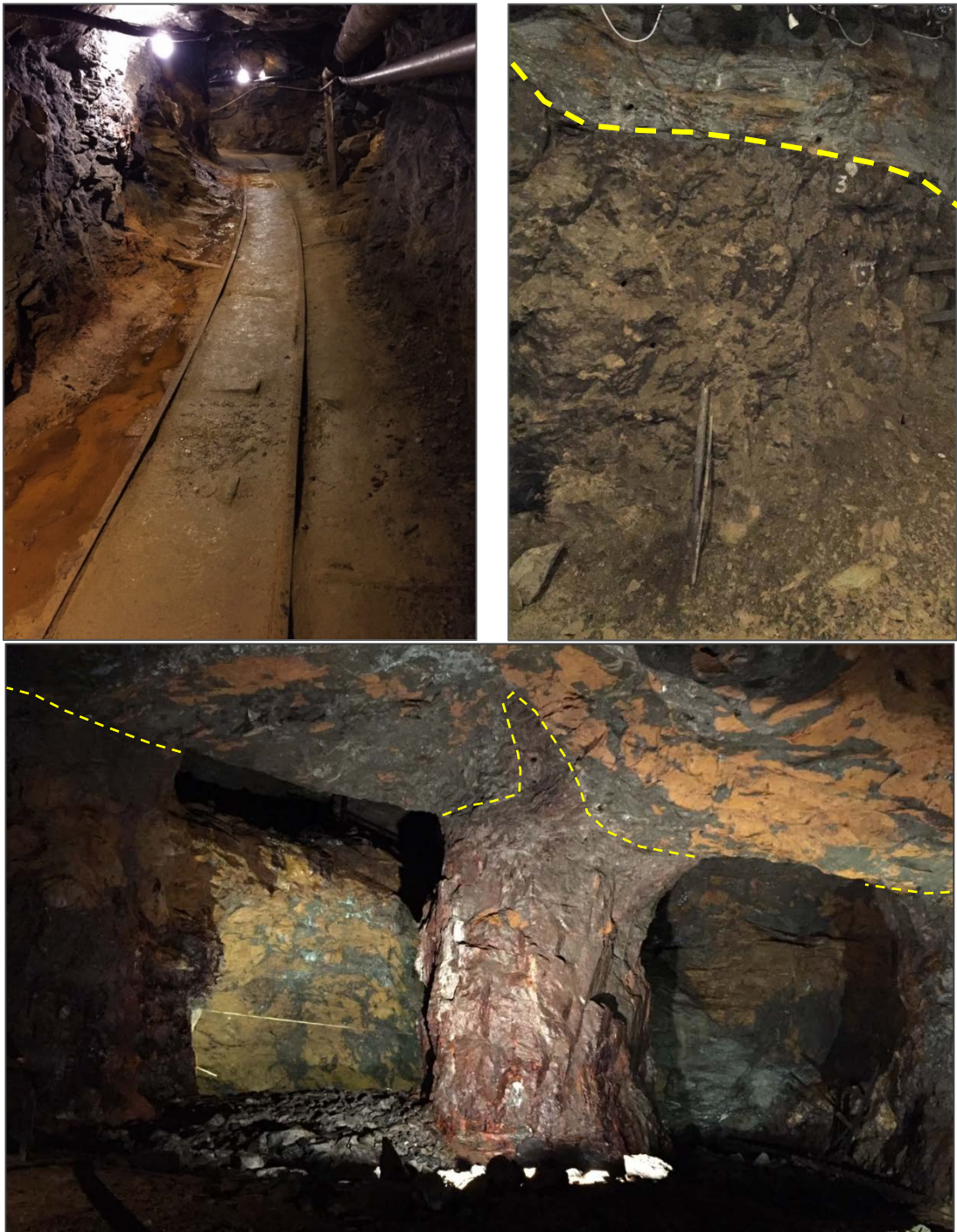
Figure 8: Photographs taken in underground workings at the Olav mine. Clockwise from upper left: underground access, mineralised-waste contact (yellow dashed line), room and pillar workings showing mineralised pillars (yellow dashed line)
