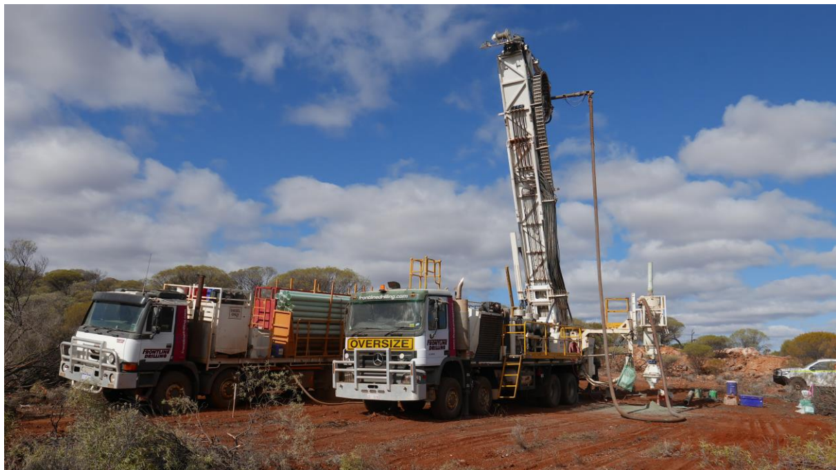
Image 1: RC percussion drilling operations at the Manindi Lithium Project
