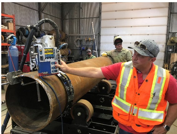
GEV pipe being welded into pressure vessels (left). David Stenning, Chief Operating Officer of GEV Canada with Finished pressure vessels for testing (right)
