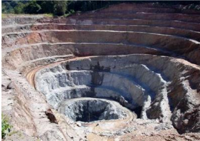
Figure 2 – Sertão Stage 5 open cut pit at the final depth of 65m.
