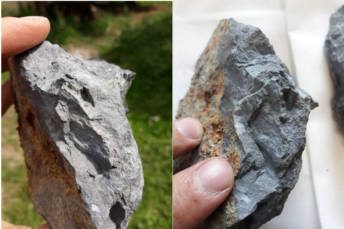
Figure 9: Samples of Massive Sulphide Mineralisation from the Gotthard Adit
