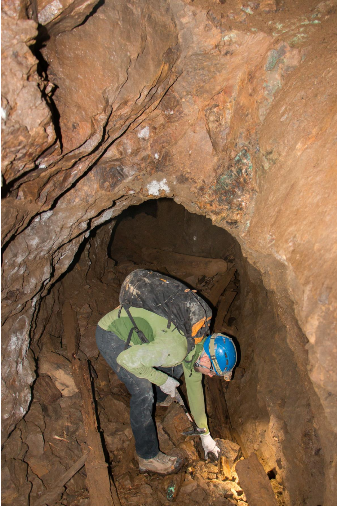
Figure 12: Exposed Copper (green malachite) mineralisation in the Langenberg Adit
