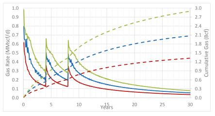
Figure 4-6: Adjusted Vertical Well type curves
