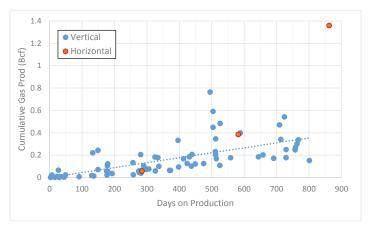
Figure 4-5: SGE pilot wells: cumulative gas vs days on production
