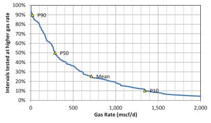
Figure 3-6: Distribution of Interval Well Test Rates
