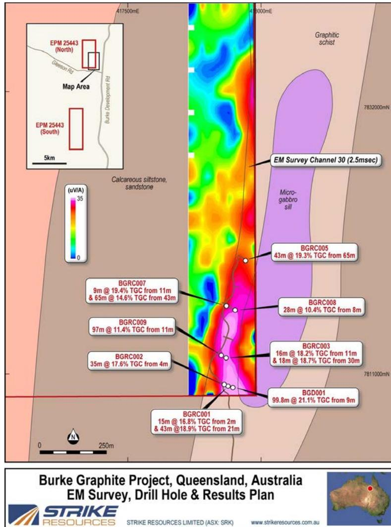
Figure 5 - EM Survey - Burke Prospect, Burke Graphite Project
