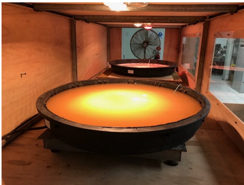
Figure 8: Brine Evaporation Trial at Bureau Veritas
