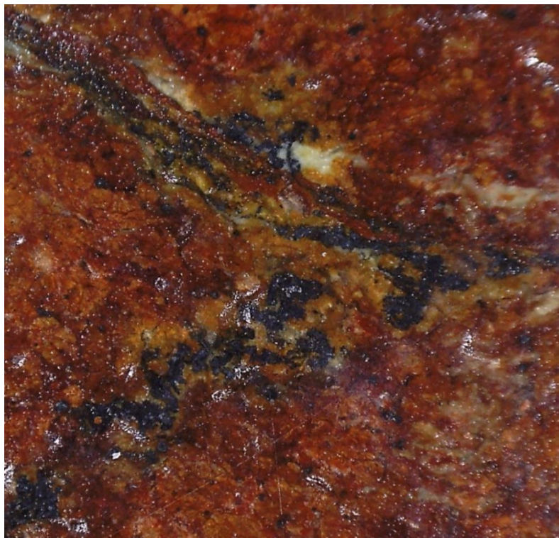
Figure 5: Photomicrograph of Polished Mt Thirsty drill core illustrating asbolane veins. Image is 4mm across.
