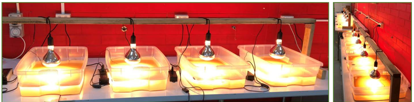
Figure 9 – Lab Based Evaporation Tests
