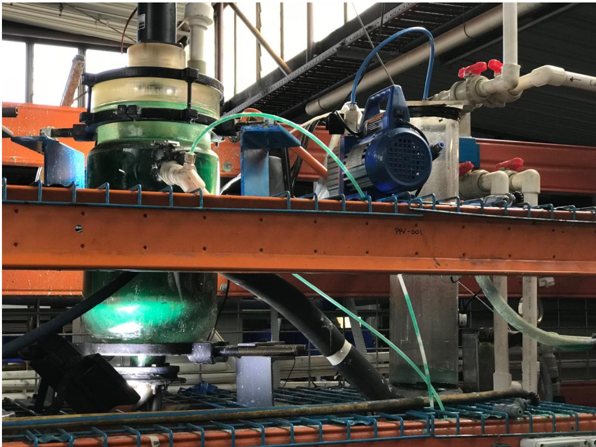
Figure 7: Crystalliser at the Company's demonstration-size processing plant, which was commissioned in conjunction with Simulus Group's laboratories.
